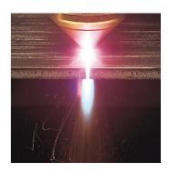
able cost since no special marking consumables are necessary. Since the marking tool is also the cutting tool, accuracy is enhanced and cycle times are shortened by eliminating tool offsets. Also, there is no reduction in machine cross-cut width associated with a separate marking station.
