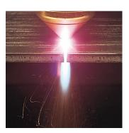
able cost since no special marking consumables are necessary. Since the marking tool is also the cutting tool, accuracy is enhanced and cycle times are shortened by eliminating tool offsets. Also, there is no reduction in machine cross-cut width associated with a separate marking station.
